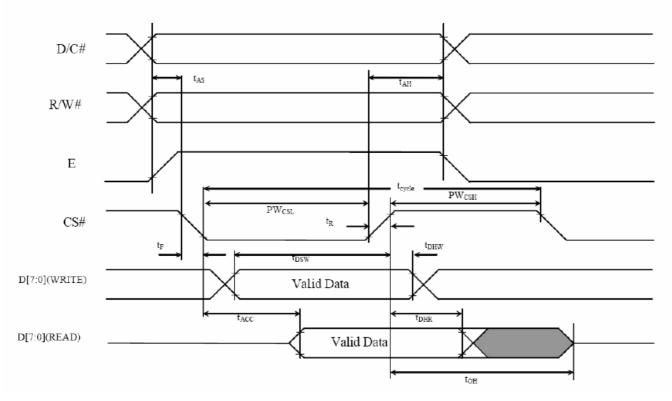
7.3.2 80XX-Series MPU Parallel Interface Timing Characteristics:
